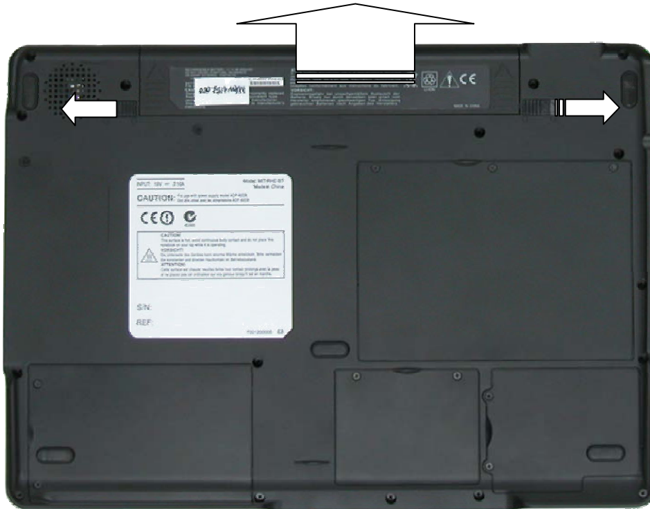
Fig. 1 Removing the battery
